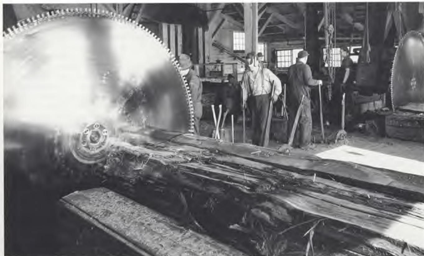
Cut-off saws prepare cedar bolts for shingle making at Vancouver's Red Band Mill. All photographs accompanying this article are from the Forest History Society archives.
